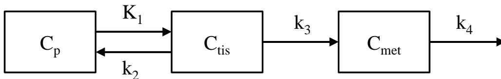
**Fig. 5.** Model used by Carson et al (1997) for analysis of [ $^{11}\text{C}$ ]raclopride plasma metabolite data. [ $^{11}\text{C}$ ]Raclopride in plasma ( $C_p$ ) exchanges with raclopride in the body pool ( $C_{\text{tis}}$ ) from which metabolites in plasma ( $C_{\text{met}}$ ) are produced. The model was further reduced by assuming  $k_4=0$  [Carson et al. 1997].
